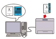
You can print two or more pages on both sides of a sheet of paper. For models with the duplexer (2150cdn Color Printer), automatic duplex printing is available. Manual duplex printing is available for models without the duplexer (2150cn Color Printer).
